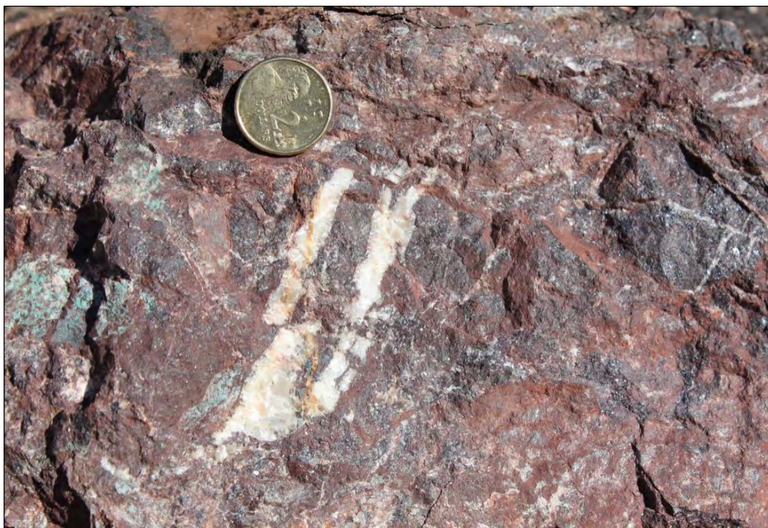
Figure 60. Typical specular haematite-quartz-carbonate alteration with secondary copper at the Old Baldy prospect.
