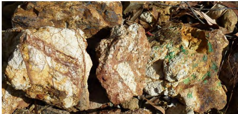
Figure 23C. Oxidised sulphide vein network with malachite in wallrock surrounding vein at Last Chance.
